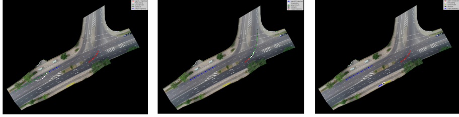
Fig. 5. Avoid the obstacle and return to the agent Trajectory. In each image, the green trajectory is the ground truth and the white is the predicted result. The black point is the sudden obstacle. The agent avoids the obstacle and returns to the original trajectory.
